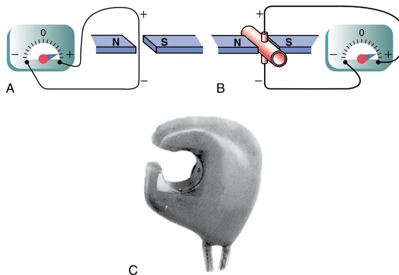
**Figure 14-4** Flowmeter of the electromagnetic type, showing generation of an electrical voltage in a wire as it passes through an electromagnetic field (A); generation of an electrical voltage in electrodes on a blood vessel when the vessel is placed in a strong magnetic field and blood flows through the vessel (B); and a modern electromagnetic flowmeter probe for chronic implantation around blood vessels (C).
